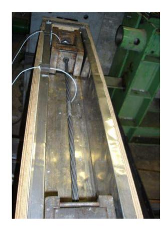
Proper stabilization criteria (e.g. waiting for a specific time, etc.) for temperature of tendon is not given!
